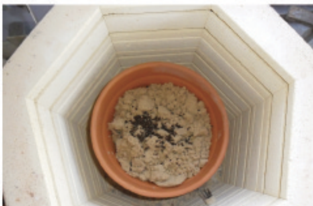
5. Ashing process in the kiln
